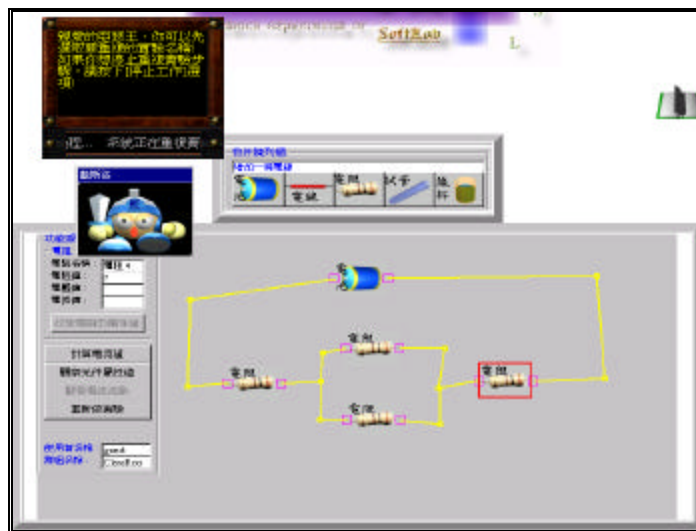
Figure 6. Virtual experiment environment of circuit experiment
