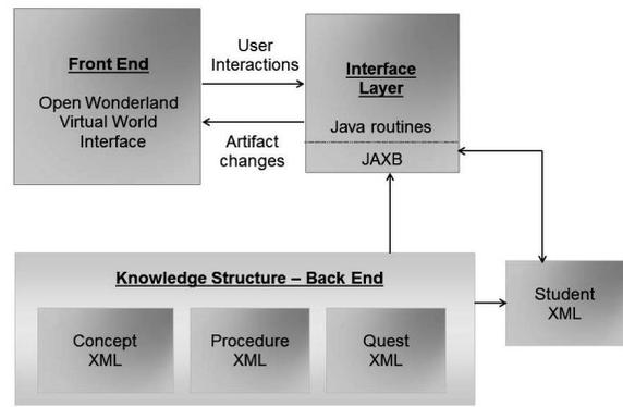
Figure 3: Architecture Diagram of vCLOT
