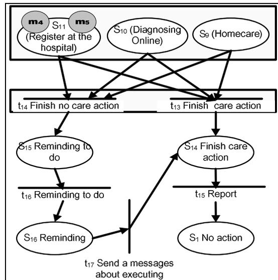
Fig. 4 Action module in Petri nets
